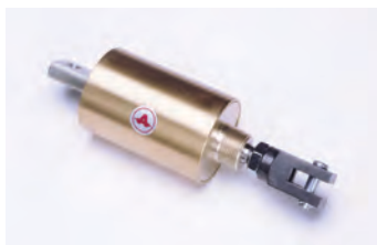
Air Cylinder Assembly No. 304 A 1 1/2" (38mm) bore, 1" (25mm) stroke air cylinder, complete mounting bracket, and clevis.
